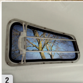
Cadre en acier inoxydable, très stable Stainless steel frame for window, very stable and stainless
